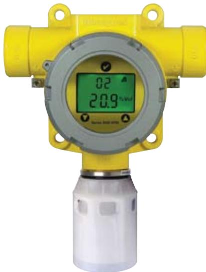
The Intrinsically Safe smart sensors are supplied pre-configured and can be 'hot swapped' without having to remove power to the detector, saving time and money during commissioning and routine servicing. A remote sensor mounting kit is available that allows the sensor to be mounted up to 50' (15m) from the transmitter, making it ideal for operation in areas that are difficult to access.
